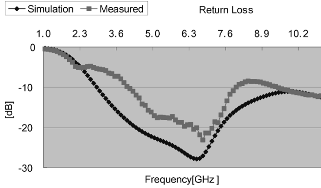
Fig. 4. Simulated and measured results of the VHDMA.
